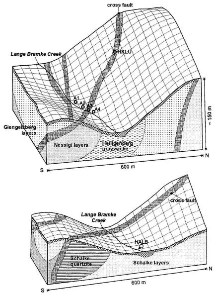
Figure 3 Simplified hydrogeological section along the fault line between the well HKLU and spring A4
